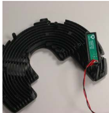
Picture 12: Positioning of the Battery Holder onto the heat exchanger
