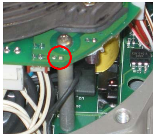
Pictures 8a and 8b: JP1 pins welding
