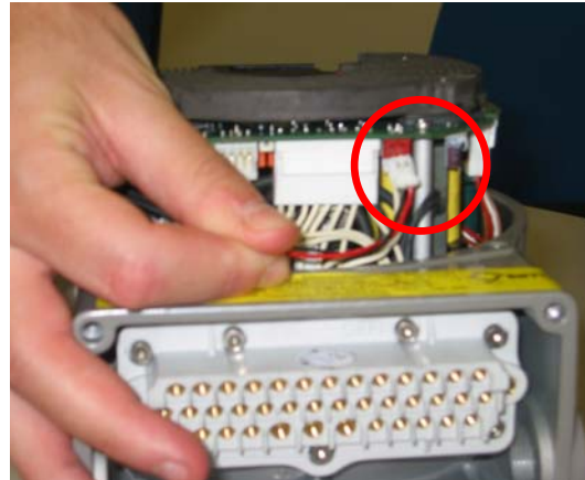
Pictures 15a and 15b: Fixing the Battery Holder onto the F02 Actuator
