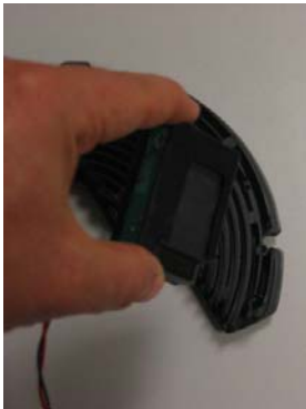
Picture 12: Positioning of the Battery Holder onto the heat exchanger
