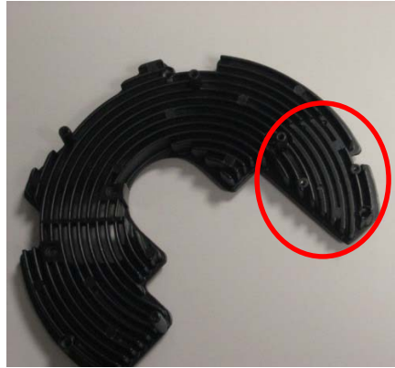
Picture 11: Position of the battery housing on the Actuator's heat exchanger
