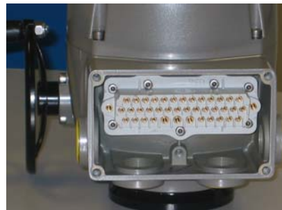
Picture 5/5a: Electrical Connections
