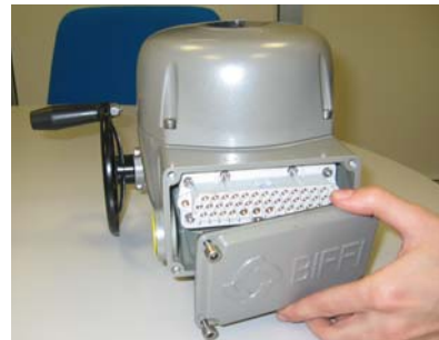
Picture 3/3a: Removing Terminal Board Enclosure
