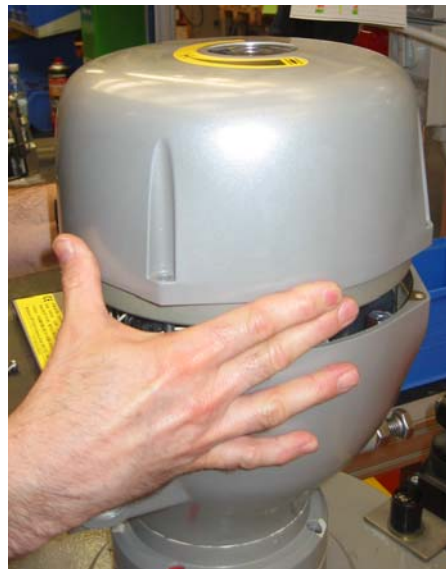
Pictures 3/3a: Removing F02 Actuator Enclosure
