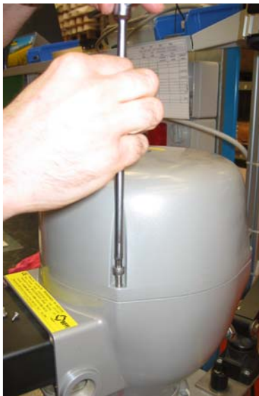
Pictures 3/3a: Removing F02 Actuator Enclosure
