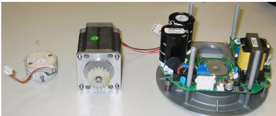
Picture 14: Motor and Position Sensor removed
