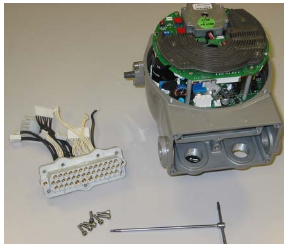
Picture 9: Actuator after the terminal board removal
