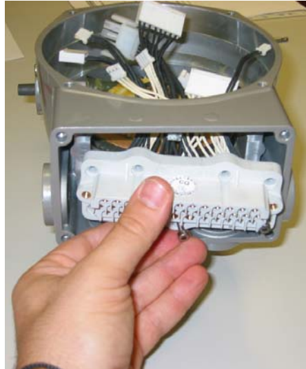
Picture 19: Replacing the terminal board onto the actuator
