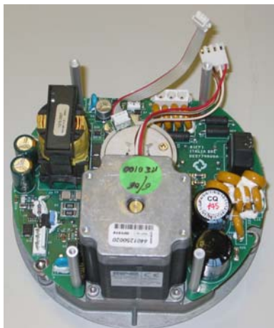
Picture 15: Electric Motor and Position Sensor Assembled onto the 3-phase card
