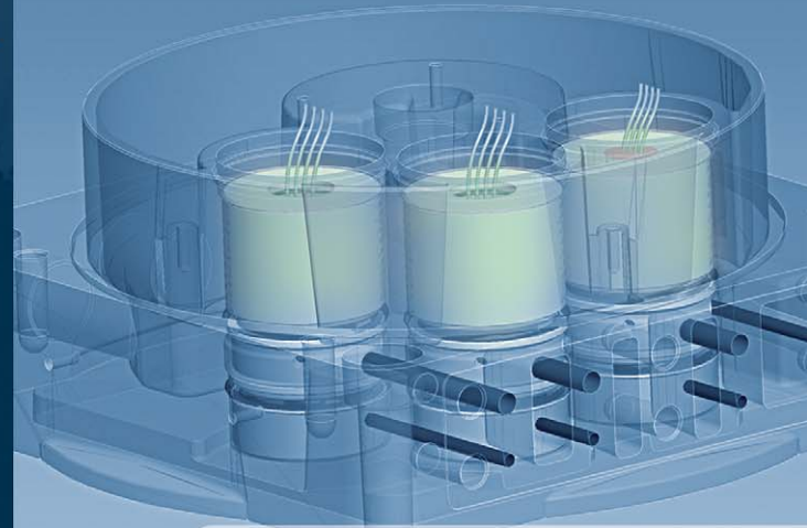
Integrated actuator and line process pressure sensors
