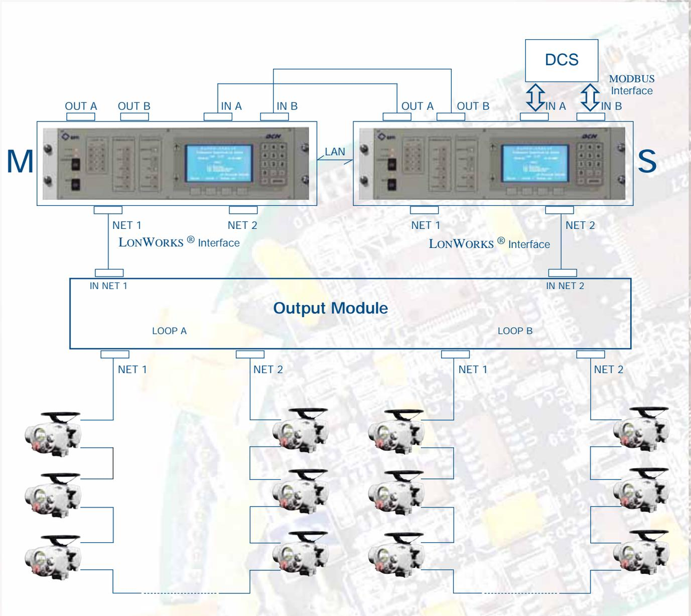
The network can comprise various loops as long as the maximum number of nodes (250) is not exceeded.
